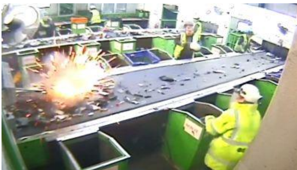
Figure 4 - Battery exploding in a recycling facility endangering employees (picture from ESA Zombie Batteries campaign/ITV News)
